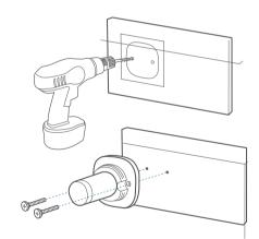
3. Firmly screw the knob of the mounting bracket into the mounting hole.
