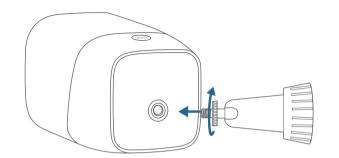
4. Hold and screw the camera to the mounting bracket. Rotate the camera to adjust the view and check it using the live stream, which you can access in the eufy Security app.
